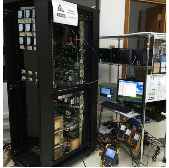
Fig. 9. Experimental setup of the TCLC-HAPF hardware prototype and its testing environment.
